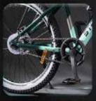
Noiseless Single Speed Freewheel & Smooth Rolling Bushless Chain Cotterless Single Speed Chainwheel
